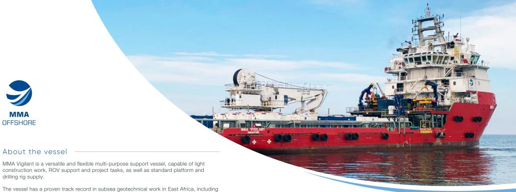
working with Benthic's PROD system in over 2,000m of water depth, deploying current meters and AUV systems and operating work class ROVs.
