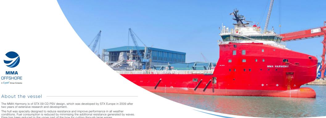
conditions. Fuel consumption is reduced by minimising the additional resistance generated by waves. Flare has been reduced in the upper part of the bow for cutting through large waves.
